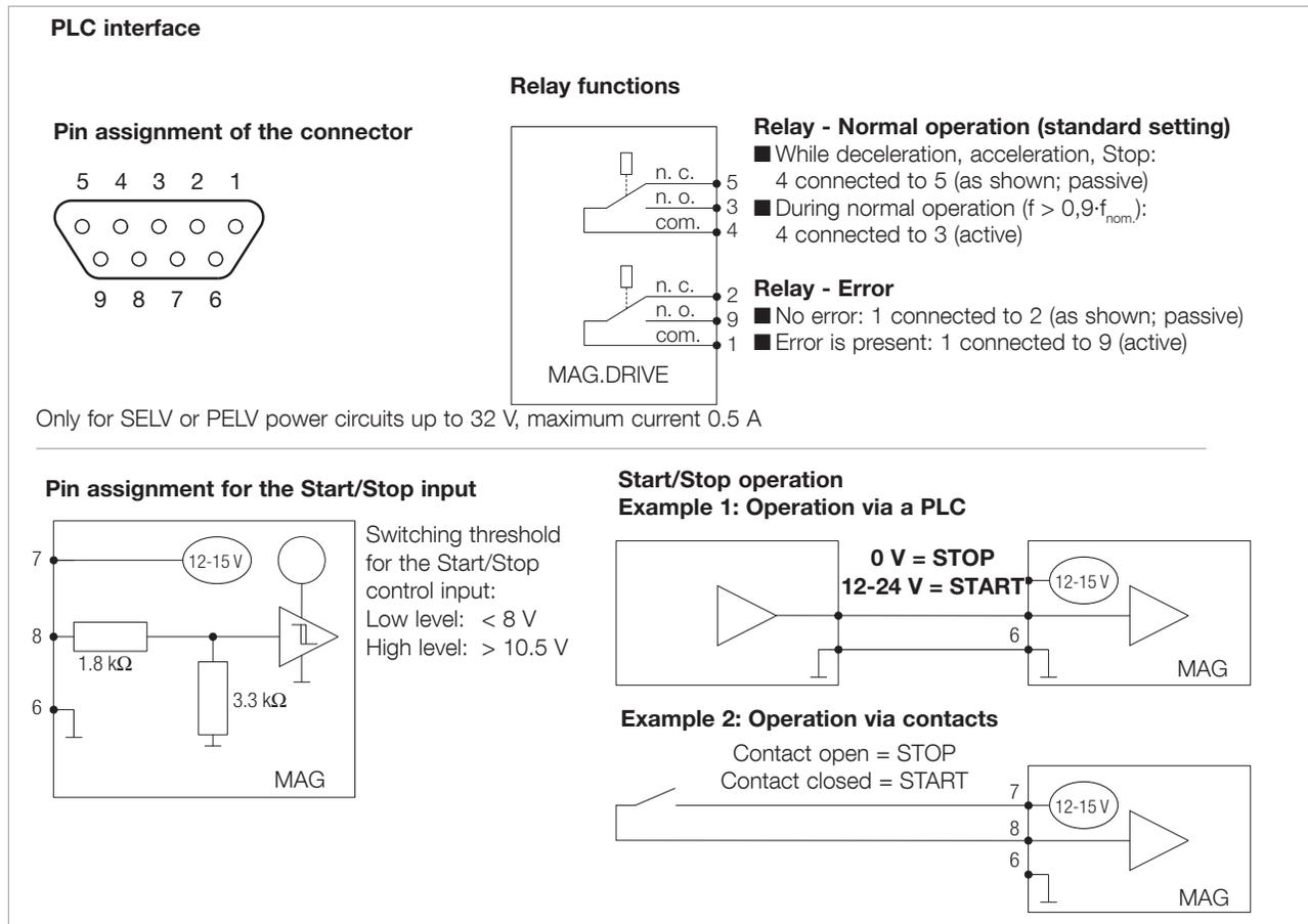
Fig.3.20 Pin assignment of the CONTROL connector
