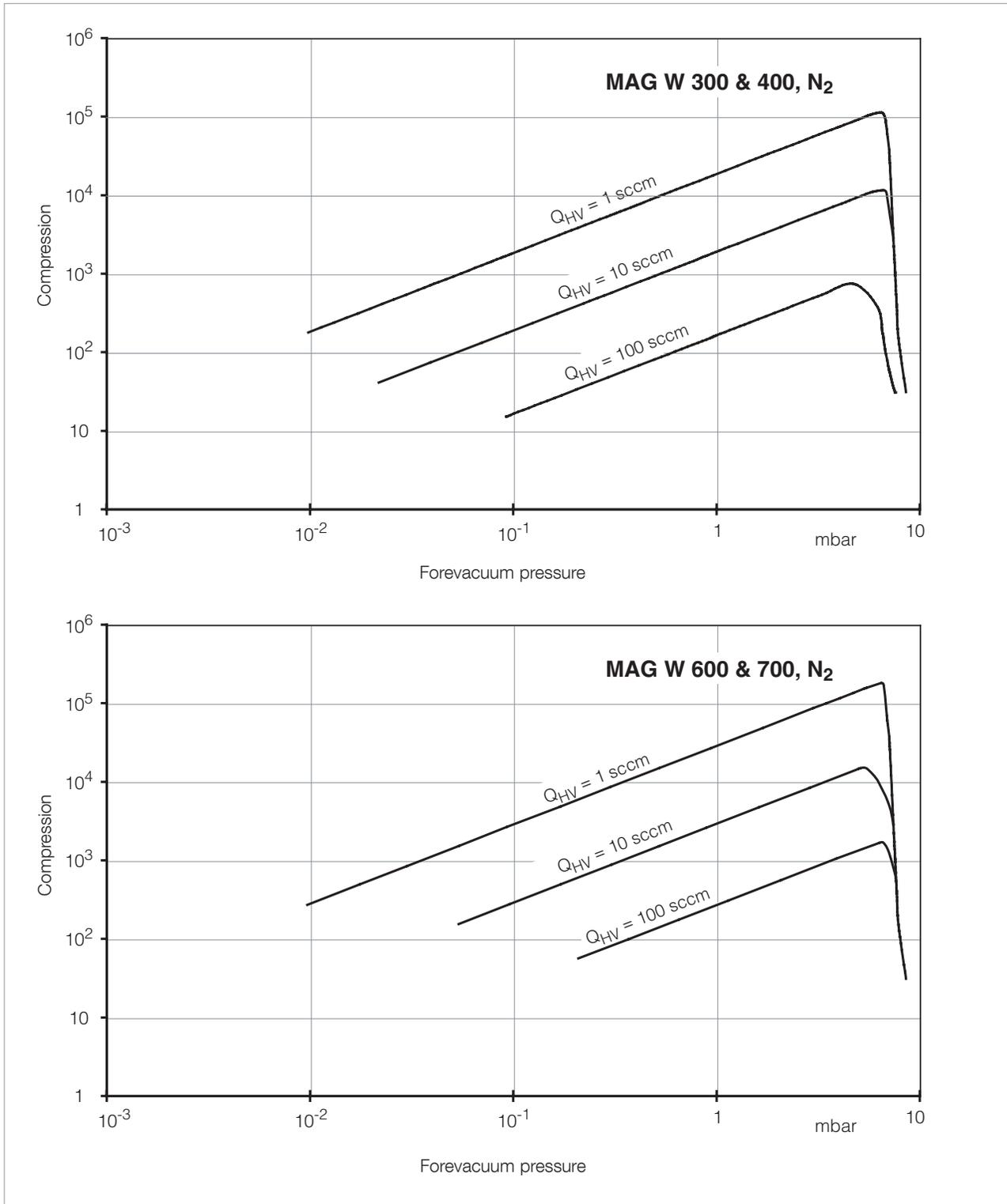
Fig. 1.5 Compression curves for Nitrogen
