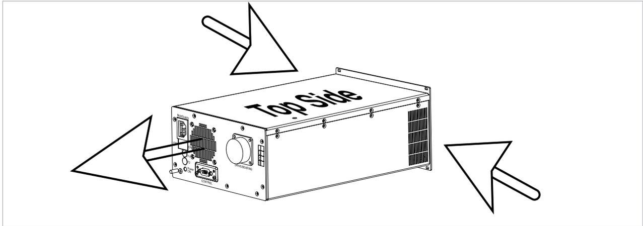
Fig. 3.19 Air flow pattern for MAG.DRIVE S
