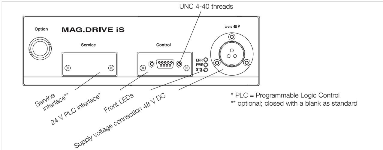
Fig. 3.15 View of the integrated frequency converter
