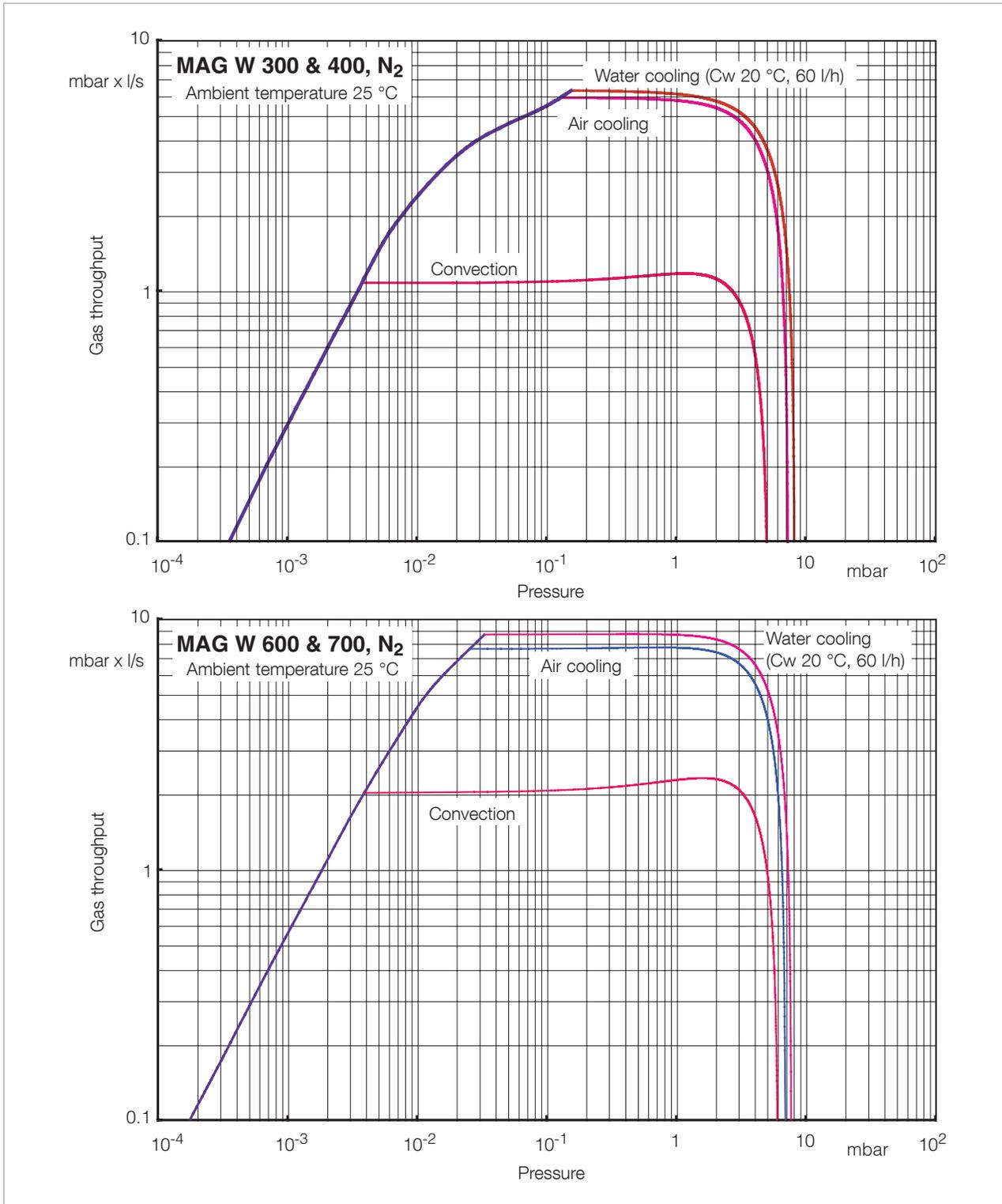
Fig. 1.7 Throughput curves for Nitrogen
