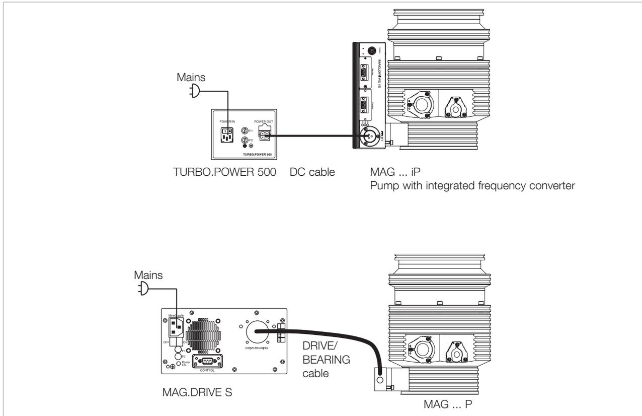
Fig. 1.11 System configurations
