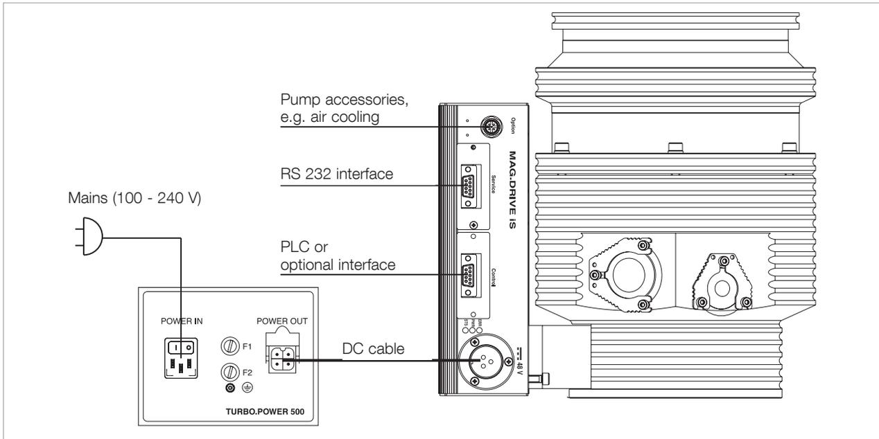
Fig. 3.14 Connection schematic TURBO.POWER 500 power supply
