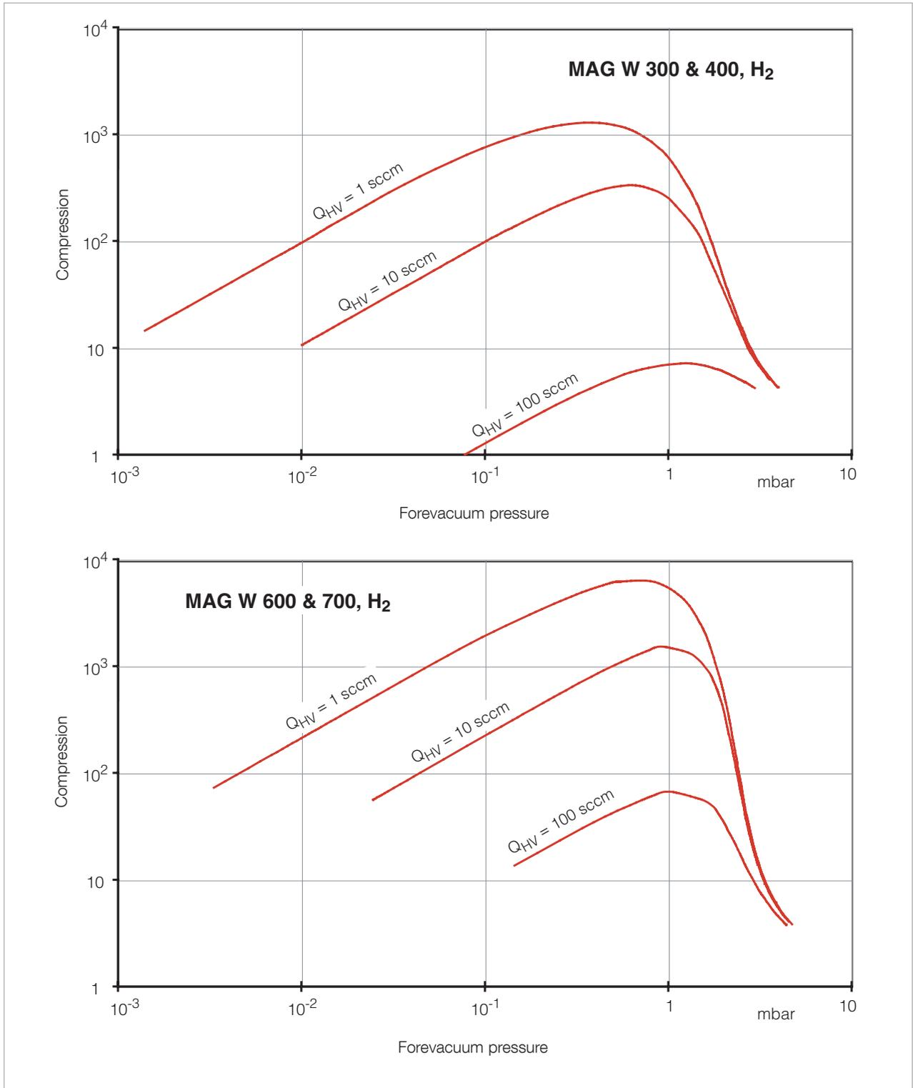
Fig. 1.6 Compression curves for Hydrogen
