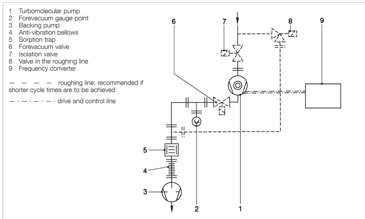
Fig. 3.8 Layout of a turbomolecular pump system
