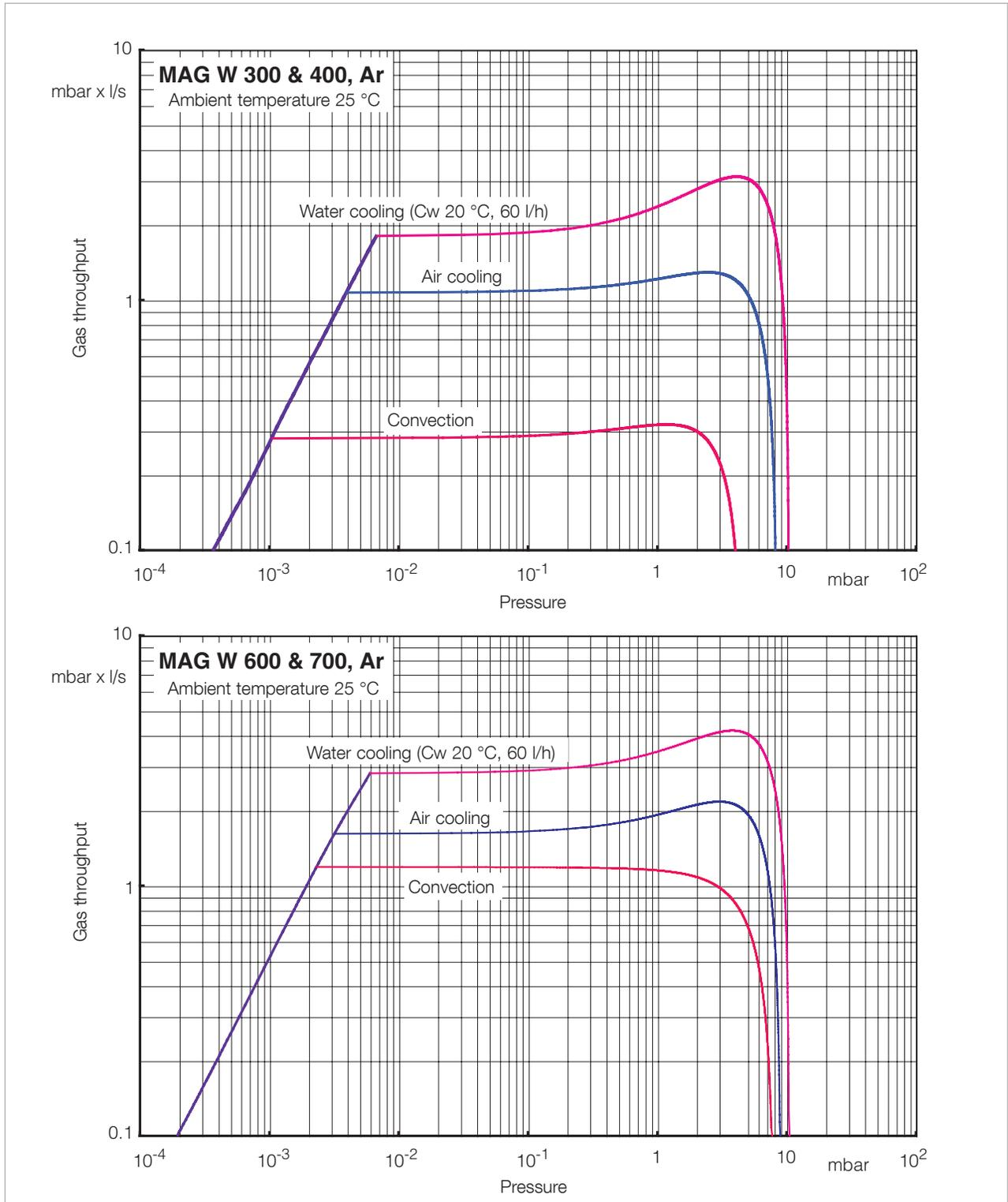
Fig. 1.8 Throughput curves for Argon
